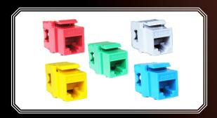
D-Link Category 5e keystone jacks are RJ45 8P 8C 50u' jacks suitable for 22-26 AWG stranded and solid wire, compatible with both 110 & Krone punch down tools. They are available in universal labels Colour coded for T568A and T568B wiring schemes and fit in high density keystone patch panel. It supports IEC 60603-7-4 and complied with ANSI/TIA EIA-568-C.2 standard.
